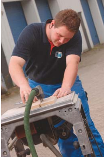
A circular saw with dust extraction above and below the sawing table
