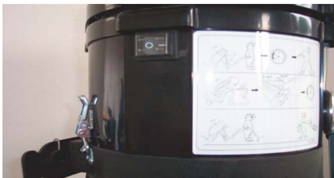
The switch should be protected against dust
