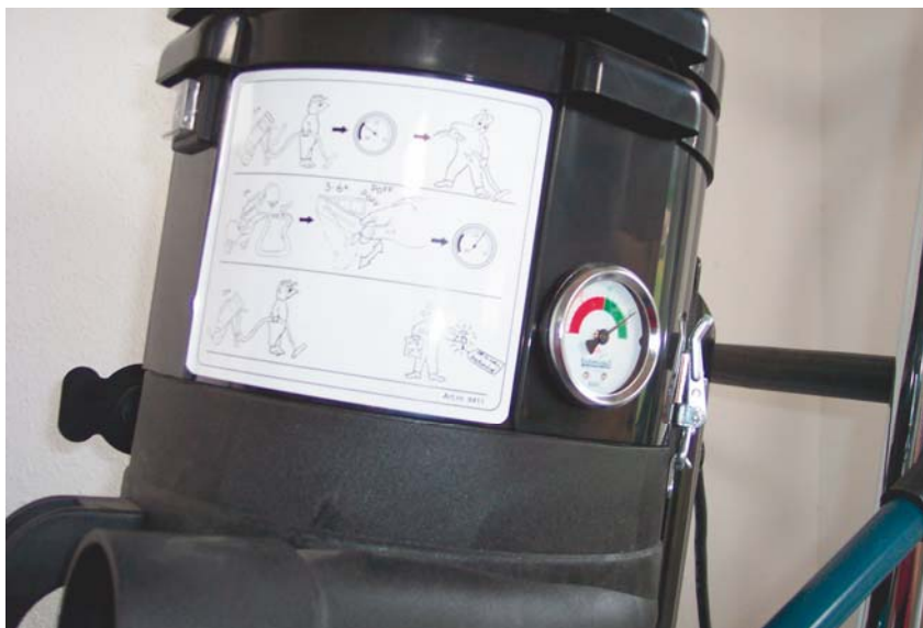
A pressure gauge indicates when the filter must be cleaned
